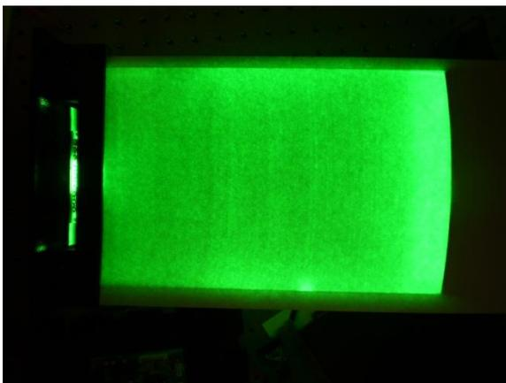
*Figure 4: Wedge backlight with 3 green LED's within 30 mm width at input and with white paper diffuser over surface*
