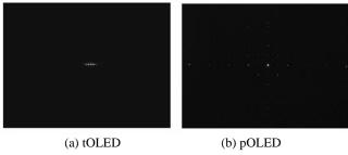
**Figure 2.** Point-spread functions through the two display panels: (a) tOLED and (b) pOLED
