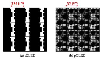
**Figure 1.** Two samples of display panels: (a) tOLED and (b) pOLED
