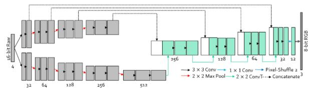
Figure 5. Network structure for Unet
