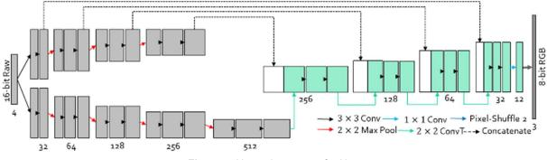
Figure 5. Network structure for Unet
