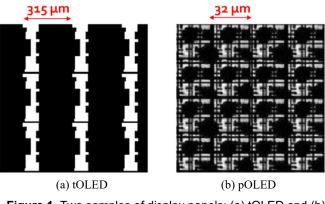
**Figure 1.** Two samples of display panels: (a) tOLED and (b) pOLED
