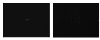
(a) tOLED (b) pOLED Figure 2. Point-spread functions through the two display panels: (a) tOLED and (b) pOLED
