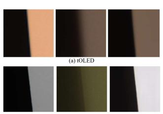
(b) pOLED Figure 3. Slant edge test for (a) tOLED and (b) pOLED: original, raw, and recovered images
