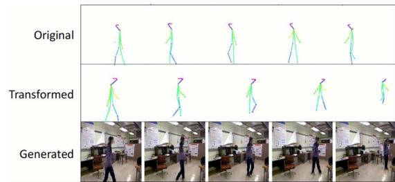
Figure 8: Perspective transform example.
