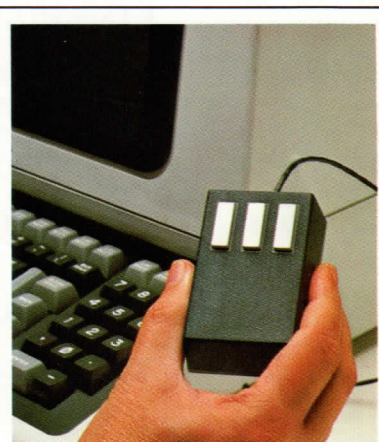
The HAWLEY X063X Mouse, a high-resolution digital input device, moves the cursor in any direction on a computer display screen, in direct proportion to its own movement.
