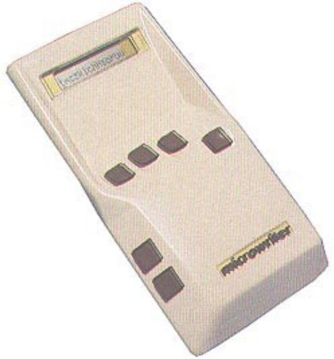
Microwriter was not really a computer, but a very original pocket word processing system, designed in 1980 by Endfield Cie in the USA and later manufactured in the UK. It used a keyboard with only 6 keys which made it possible to keyboard all the alphabet letters, numerals and punctuation marks. The typing method used the letters shape likeness and only one hand was necessary to type text. It only required a few hours to get used to keyboard and then typing speed could be very fast.
