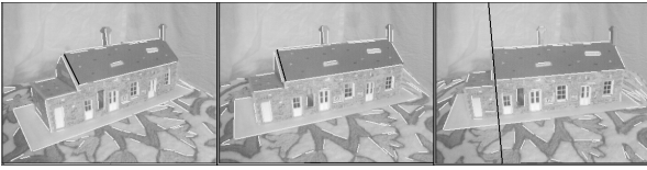
Figure 6: Trifocal line transfer. Corresponding lines in the first two images (the roof edge marked in black) predict the infinite line in the third.
