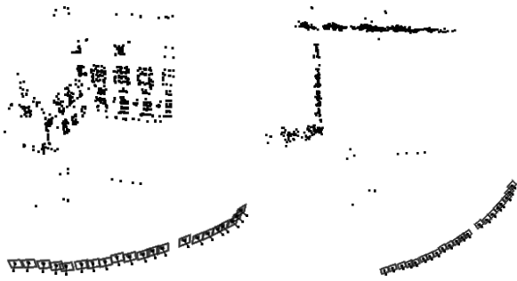
Figure 11: Castle : Computed cameras and 3D point structure. The plan view shows the accuracy of the self calibration.
