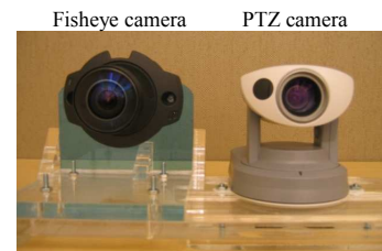
Fig. 1. The camera combo hardware.
