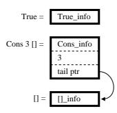
Figure 7.2: Heap Representation of Constructed Values
