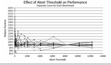
Figure 12.21: Performance Effect of Adjusting the *MAXBLAME* Tunable—geometric mean
