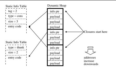
Figure 7.1: Structure of Heap Closures
