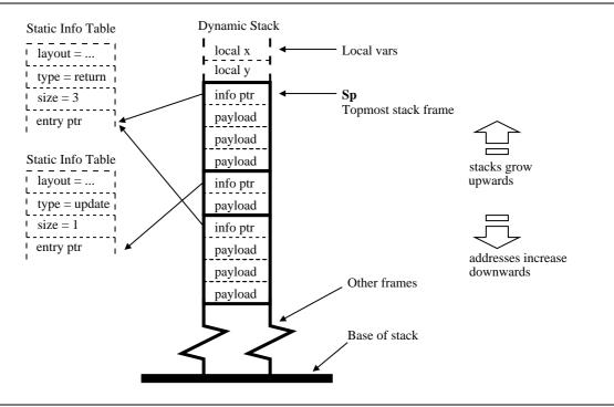
Figure 7.6: Structure of Stack Frames
