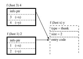
Figure 7.4: Heap Representation of Thunks
