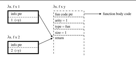
Figure 7.3: Heap Representation of Functions
