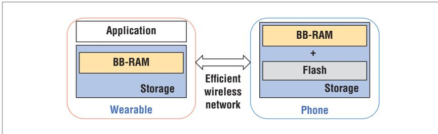
Figure 4. The WearDrive architecture. Essentially, WearDrive exploits the battery in a nearby phone to provide durability for the data in the wearable’s “battery-backed” RAM (BB-RAM) storage.
