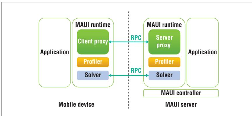
Figure 6. The MAUI (Mobile Assistance Using Infrastructure) architecture. The runtime on the phone dynamically determines if it is more power efficient to offload a function call to the server. The server could be a nearby device or in the cloud.
