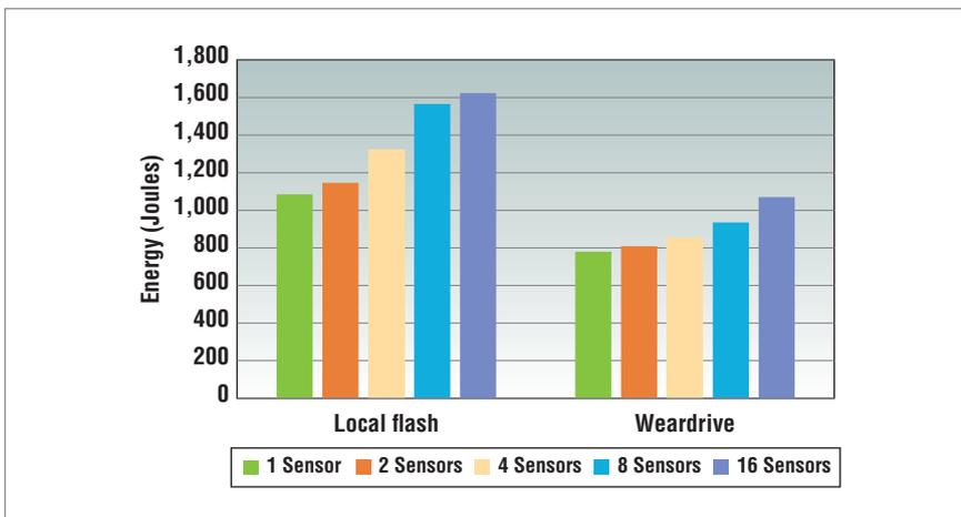
Figure 5. Energy used when storing to local flash memory vs. using WearDrive, based on between 1 and 16 sensors generating data continuously at 1 Hz for 24 hours. A typical smartwatch battery stores between 3000–6000 Joules of energy.
