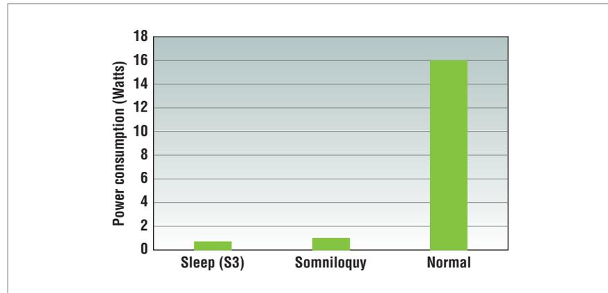
**Figure 2.** Power consumption of a Lenovo X60 using Somniloquy. Somniloquy provides increased functionality of filtering network packets that is not possible in the S3 sleep state, even when wake-on-network is available. The power saving compared with supporting the same functionality on the main CPU is significant.
