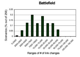
**Figure 1**. Distribution of number of scenario files according to number of topology changes during 900-second simulation.
