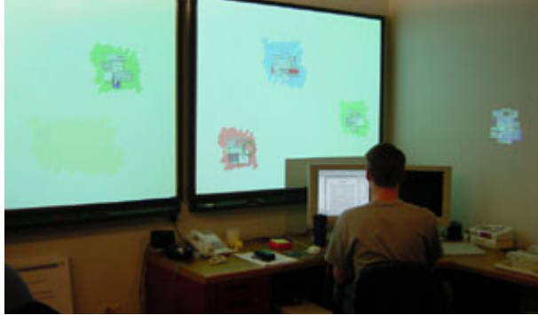
Figure 2.3. Kimura presents interactive montages of images on large peripheral displays to help users manage multiple working tasks.
