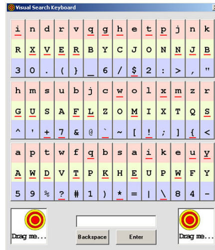
Figure 5.4. The Spy-Resistant Keyboard. . In the first phase of typing, the mapping phase, the user must first find the character they would like to type and note its location. For example, if they are trying to type the capital letter “Z”, they would scan the three green rows, finding the letter on the seventh tile on the second row.
