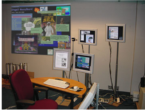
Figure 1.2. The Display Garden, a rapidly configurable collection of physical display devices such as whiteboards, pin-up space, audio displays, mobile LCD panels, and large projection surfaces on various surfaces in the room.
