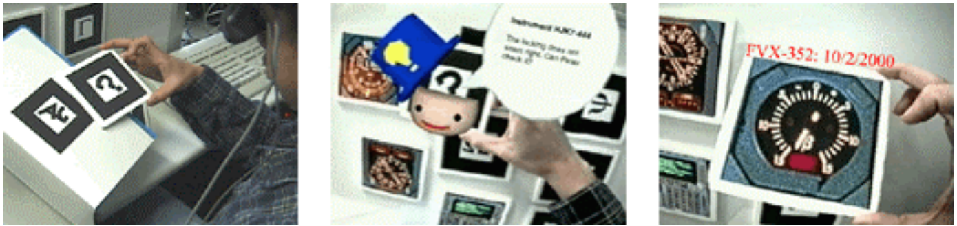
Figure 1: (a) Physical manipulation of help and data cards; (b) User view: Moving help card beside data card to acquire Tangible Bubble Help; (c) User view: Tilting physical card to attain Tangible Tooltips on virtual instrument.
