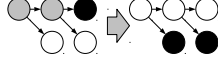
Figure 4: Dispersive symbolic execution preprocessing. The black dispersive target on the left is converted to two convergent ones on the right using a reverse control-flow analysis (gray).
