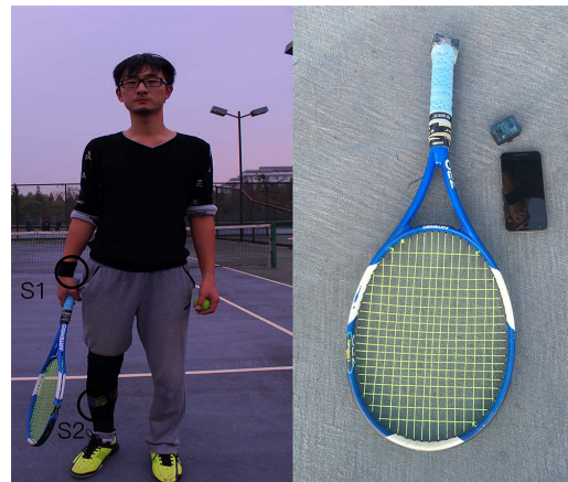
Figure 1: An application scenario of TennisMaster through the IMU sensors mounted on the bottom of racket and the shank of user with smartphone controlling.
