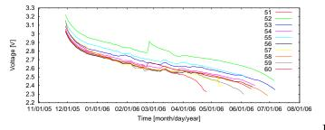
Figure 13: Supplied battery voltage for the motes in the Olin deployment. The supplied voltage is averaged over one day.
