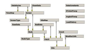
Figure 4: Sensor Network Database Schema. The different boxes correspond to database tables, while the arrows correspond to relations between tables.
