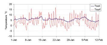
Figure 10: Air and soil temperature over six weeks. Each point represents six hour averages. Tsoil: soil temperature at 10 cm depth; Tsurf: air temperature at soil surface.
