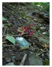
(b) Mote inside its waterproof enclosure deployed in the field.
