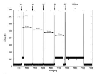
(b) The average current draw during the 0.79 seconds of sampling sensors S1 to S5 is 0.64 mA. Considering 60 seconds between successive sampling rounds, the average current drawn by this process is 0.008 mA.
