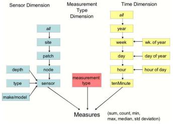
Figure 6: Sensor data cube dimension model.
