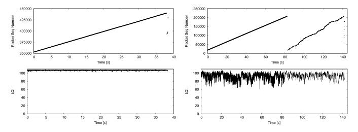
Figure 16: Two examples of data downloads. The graphs on the left correspond to a download over a high-quality wireless link while the ones to the right correspond to a transfer of the same amount of data over a lossy link.
