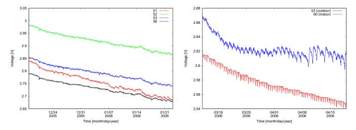
Figure 14: Voltage over time for two different periods: winter (left) and spring (right).
