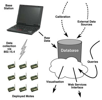
Figure 1: Architecture of the end-to-end data collection system.
