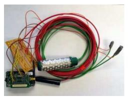
(a) MicaZ mote with attached data acquisition board and soil moisture and temperature sensors.
