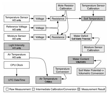
Figure 5: Calibration workflow converting raw to derived science data.
