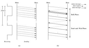
Figure 3: Status report protocol (a) and download protocol (b). The Receiving timeline on the left illustrates the time that the mote's radio is turned on (2 sec) and the total cycle time (2 min).
