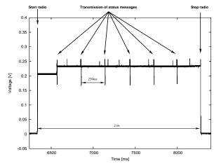
(a) The average current draw during the 1.9 seconds of radio activity is 22.922 mA. Considering that the radio is turned off during the remaining 118 seconds of the report interval, the average current drawn by the radio is 0.36 mA
