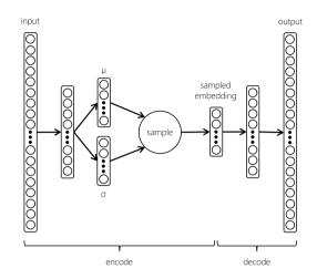
Figure 6.6: Instead of directly generating an encoded representation, variational autoencoders sample the latent vector from the generated vector of means  $\mu$  and standard deviations  $\sigma$ . This local variation forces the model to learn a smoother and more continuous latent space.
