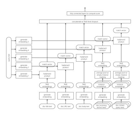
Figure 7.5: A neural architecture for ranking documents with multiple document fields. A new latent space is learnt—corresponding to each field—and the query and the document are compared in each of these latent spaces to generate a match vector. The relevance of the document to the query is estimated by aggregating the matching signals across the different latent spaces.
