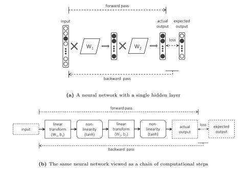
Figure 6.1: Two different visualizations of a feed-forward neural network with a single hidden layer. In (a), the addition of the bias vector and the non-linearity function is implicit. Figure (b) shows the same network but as a sequence of computational nodes. Most neural network toolkits implement a set of standard computational nodes that can be connected to build more sophisticated neural architectures.
