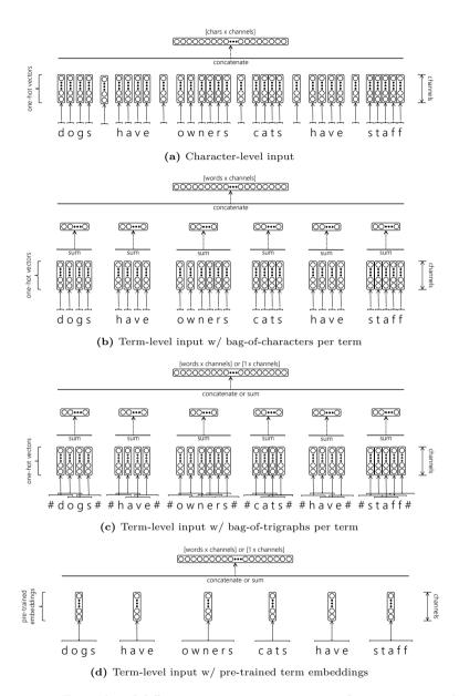
**Figure 6.3:** Examples of different representation strategies for text input to deep neural network models. The smallest granularity of representation can be a character or a term. The vector can be a sparse local representation, or a pre-trained embedding.
