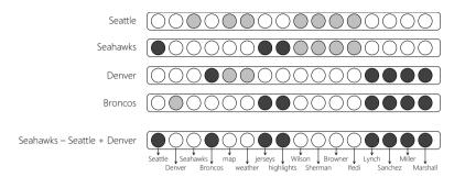
**Figure 3.5:** A visual demonstration of term analogies via simple vector algebra. The shaded circles denote non-zero values. Darker shade is used to highlight the non-zero values along the vector dimensions for which the output of  $\vec{v}_{Seahawks} - \vec{v}_{Seattle} + \vec{v}_{Denver}$  is positive. The output vector is closest to  $\vec{v}_{Broncos}$  as shown in this toy example.
