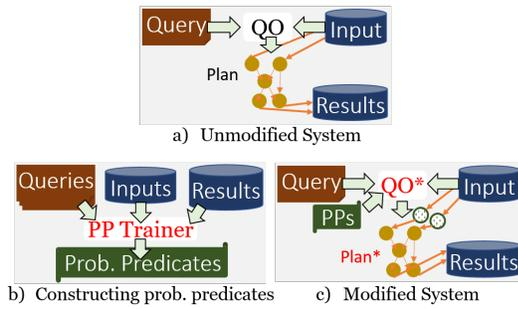
**Figure 3:** Comparing the unmodified query processing system on the top with the proposed system on the bottom. Key changes are in the training and use of probabilistic predicates (PPs). See [13] for details.
