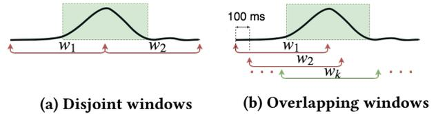
**Figure 4: Striding Windows—  $w_1$  and  $w_2$  are disjoint windows in (a), while they are overlapping in (b)**
