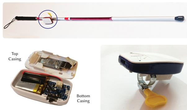
Figure 1: GesturePod. Top image shows the pod attached to a white cane. Bottom left image shows the interior of the pod.
