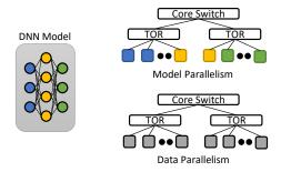
Fig. 2. A DNN model is partitioned across multiple nodes in a modelparallelism case, and the whole model is replicated in the data-parallel case.
