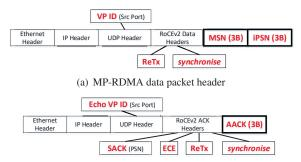
(b) MP-RDMA ACK packet header
