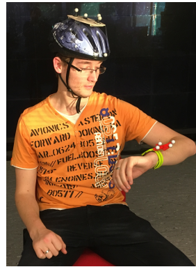
Fig. 2. Left: A participant, wearing helmet and smartwatch both with markers attached, is reading a text displayed on the smartwatch while sitting. Right: Measurements taken during the pre-study.
