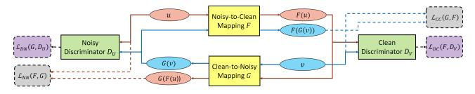
Figure 2: The architecture of ACSE. Forward and backward cycles are shown in red and blue lines respectively. Noisy and clean training features U and V are unparalleled. Identity-mapping losses  $\mathcal{L}_{IN}(G)$  and  $\mathcal{L}_{IC}(F)$  are not shown in this figure.
