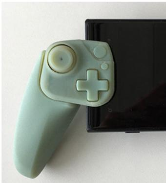
**Figure 2:** The two wireless units may be removed from the charging dock and clipped to a mobile device such as a smartphone to support mobile gaming.
