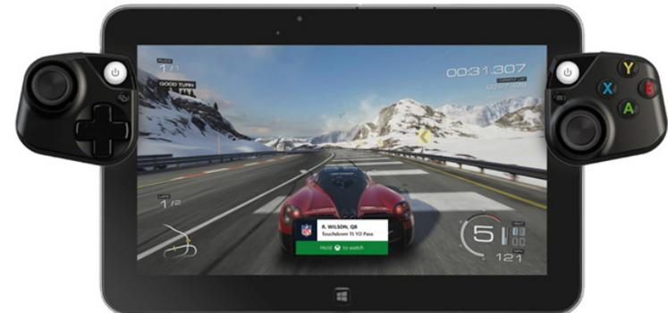
The left- and right-hand parts of the mobile controller are independent Bluetooth low-energy (BLE) devices, each with their own BLE microcontroller and battery. A docking station which connects to exposed contacts inside each clasp mechanism allows for recharging. The triggers are based on force-sensing resistive (FSR) material and are auto-calibrated.
