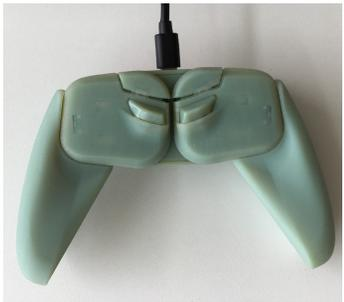
**Figure 4:** Trigger and bumper controls are located on the underside of the controllers.
