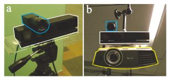
Figure 2. (a) Our Hybrid HFR Depth uses off-the-shelf Point Grey camera and Kinect v2. (b) Our projection mapping system adds an off-the-shelf projector.
