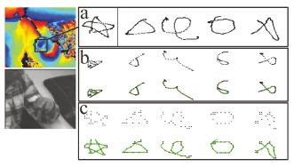
Figure 9. The user may draw simple shapes in the air to control a remote interface. (a) shows fingertip trace captured by Hybrid HFR Depth, with Kalman Filter applied. (b) is the same motion captured by Kinect, with Kalman Filter applied.
