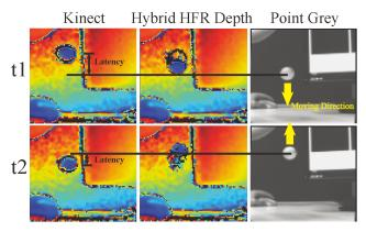
Figure 8. A ping pong ball is tracked with both Kinect v2 and Hybrid HFR Depth. The Hybrid HFR Depth image exhibits lower latency than Kinect. The high frame rate depth image is far ahead of the Kinect image but is slightly behind the Point Grey image (due to computation time).
