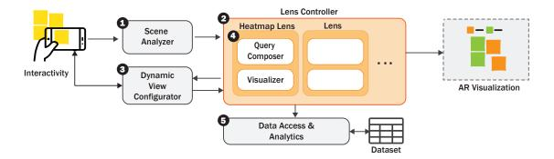
Figure 5: System Architecture. (1) Scene analyzer extracts notes from camera feed, (2) lens controller determines set of lenses applicable to notes in view, (3) dynamic view configurator updates the interface with available lenses, (4) lens queries for data from the (5) Data access and analytics module, and renders the augmented visualization.
