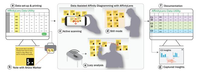
Figure 3: Affinity Lens workflow. Data is acquired (a) and automatically tagged for a Marker (b) for printing. Various forms of DAAD (c, d, e) can be documented (f) along with associated insights (g).
