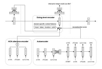
**Fig. 1**. The architecture of AE-HCN which is the same as HCN except for the autoencoder component.
