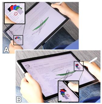
Figure 3. In bimanual grips, using either thumb is plausible. So the user can just physically tip the tablet to slide the Tools to the left or right, resolving the ambiguity.
