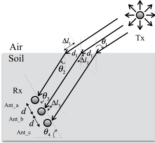
**Figure 3: Model of plane wave propagating through air-to-soil surface. Transmit and receive antennas are oriented perpendicular to the plane of the paper. The wave that travels to antenna B has a delay of  $n\Delta l_2/c + n\Delta l_3/c - \Delta l_1/c$  relative to the wave travels to antenna A.**
