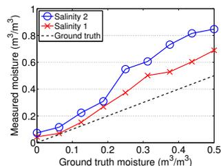
**Figure 10: Soil moisture measured by soil sensor at two salinity levels. The sensor reports higher moisture values at the higher salinity level.**
