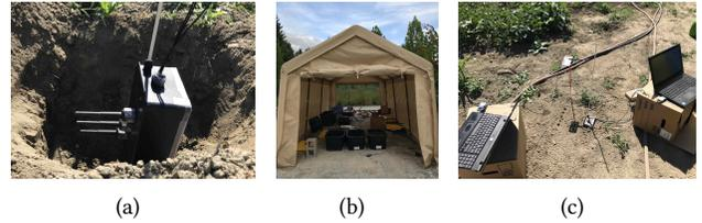
**Figure 6: Soil measurement setup for multi-antenna system.** Antennas are at different depths in soil while there is a rod coming out from soil surface to indicate the location of antenna array in soil. (a) Receive antenna array on a waterproof box. (b) Tent with soil boxes. (c) Measurement setup on a farm.
