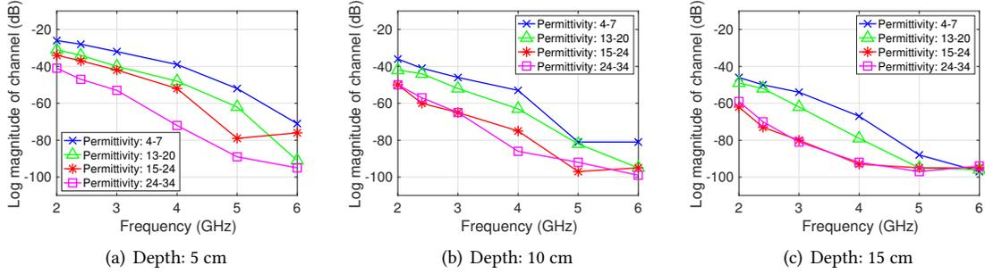
**Figure 5: Channel attenuation in soil at different depths measured by network analyzer. Generally, signal attenuation increases as frequency, depth, or soil moisture increases.**
