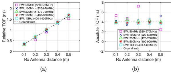
**Figure 7: Strobe’s joint relative and absolute ToF estimation performance over the air. (a) Relative ToF: Using 3 antennas to jointly estimate relative ToF and absolute ToF gives very accurate results even with a small bandwidth. (b) Absolute ToF of the antenna closest to the transmit antenna: Absolute ToF deviates more with smaller bandwidths.**
