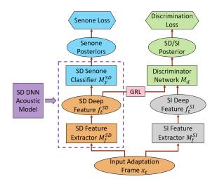
**Fig. 1.** The framework of ASA. Only the optimized SD acoustic model consisting of  $M_f^{\text{SD}}$  and  $M_y^{\text{SD}}$  are used for ASR on test data.  $M_f^{\text{SI}}$  is fixed during ASA.  $M_f^{\text{SI}}$  and  $M_d$  are discarded after ASA.
