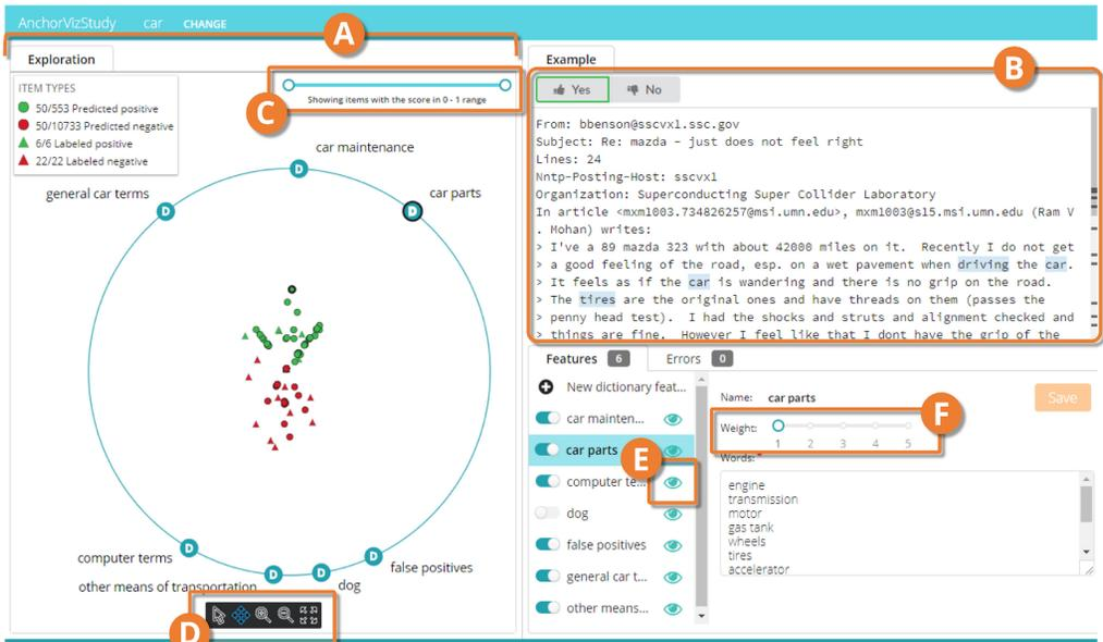
Fig. 8. The Visualization interface contains the Exploration pane on the left that hosts the AnchorViz (A) with a range slider to filter the items based on their prediction scores (C) and a zoom and pan control bar (D). The Example pane (B) displays the content of the selected item. An anchor can be shown or hidden from the visualization with the eye toggle button (E), and its weight can be updated using a slider (F).
