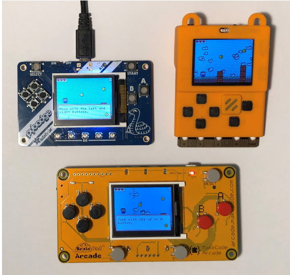
Figure 2. Three microcontroller-based game handhelds with 160x120 color screens. These boards use ARM’s Cortex-M4F core: the ATSAM51G19 (192kB RAM, running at 120Mhz) and STM32F401RE (96kB RAM, running at 84Mhz).
