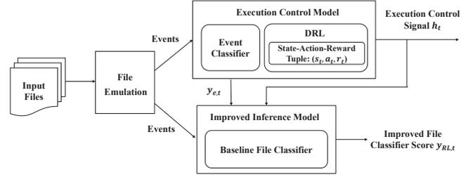
Fig. 1: Deep reinforcement learning system for halting the execution of an unknown file and improved malware classification.
