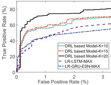
Fig. 7: Comparison between the proposed DRL-based model for  $K \in \{10, 15, 20\}$  and the best two baseline file classifiers.
