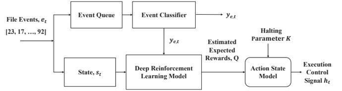
Fig. 2: Details of the execution control model in Figure 1. In both figures, the input is  $e_t$ , and the outputs are  $h_t$  and  $y_{e,t}$ .
