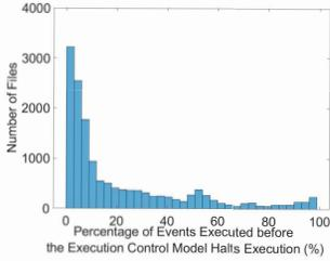
Fig. 5: Histogram of the percentage of behavioral events which are executed before the execution control model halts emulation compared to the number of executed events determined by the engine’s heuristics.
