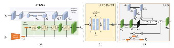
Figure 3: AEI-Net for the first stage. AEI-Net is composed of an Identity Encoder, a Multi-level Attributes Encoder, and an AAD-Generator. The AAD-Generator integrates informations of identity and attributes in multiple feature levels using cascaded AAD ResBlks, which is built on AAD layers.
