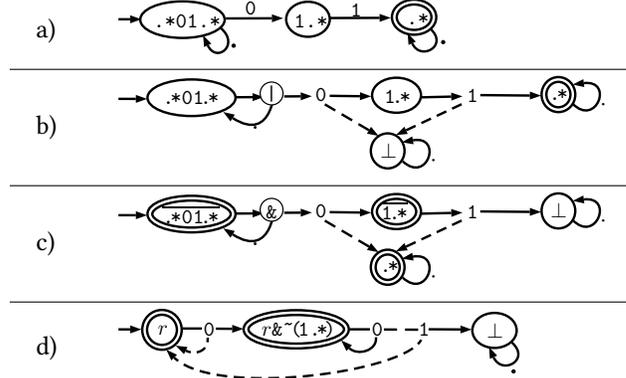
Fig. 2. a-c) Symbolic derivations viewed as transitions between regexes; d) DNF form of (c) where  $r = \sim(. * 0 1 . *)$ .
