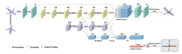
Figure 1: Overview of our multiresolution-instance-discrimination (MID) unsupervised pre-training pipeline. An augmented input point cloud via transformations is fed into the deep neural network which maintains and fuses multi-scale resolution feature maps. The shape-level features and point-wise features are extracted from the network, and they are encouraged to be discriminative and transformation-invariant under the supervision of the MID loss on both shape instance and point levels.
