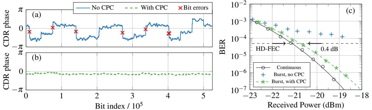
Fig. 3. Adaptive CDR phase in RxA when receiving burst mode data (a) without, and (b) with clock phase caching (CPC) enabled. Bit error locations are shown as crosses. (c) Associated BER curves.
