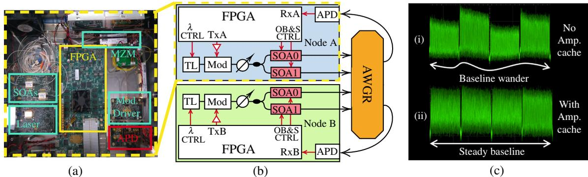
Fig. 2. (a) Space- and wavelength-switching node. (b) Two nodes perform fast OCS connections by switching the TL wavelength and active SOA. (c) APD output in Node B (i) without and (ii) with amplitude (Amp.) caching applied. Each burst represents a unique wavelength/SOA state from both TxA and TxB.
