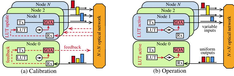
Fig. 1. Concept of amplitude caching applied to a flat  $N \times N$  optical network. (a) The optical loss of all intra-connections are pre-calibrated and cached in a lookup table (LUT) in each node. (b) During normal operation, nodes vary their launch power using the LUTs to optically equalise the received signal.
