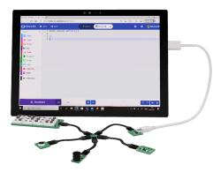
Fig. 1. A conceptual vision of a BVI accessible physical computing environment, showing a web-based accessible programming editor and hardware modules connected together by a reversible, low-cost multi-wire cable. Modules include: a braille display module, a sounder module for audio output, a haptic module for vibrational feedback, an accelerometer for orientation detection, and a re-programmable microcontroller module that controls operation of all other modules.
