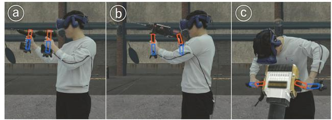
**Figure 13: GamesBond applications rendering different grip shapes: a pair of separate electric screwdrivers with independent handles (a); a hammer drill with parallel handles (b); and a jackhammer with aligned handles (c).**
