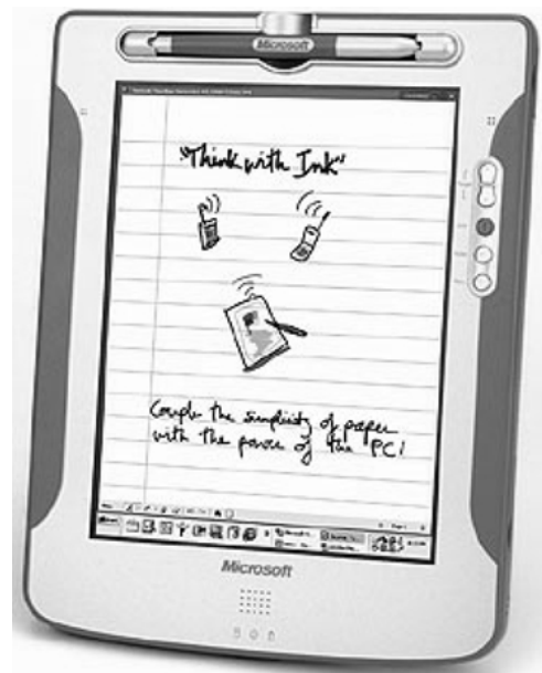
Figure 4. Prototype Tablet PC hardware with buttons on the right side that can be configured for push-to-talk.
