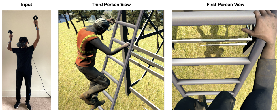
Fig. 10. CoolMoves uses limited input of the user’s hands and head to recover plausible legs motions as showcased in this scene of a user climbing a ladder.
