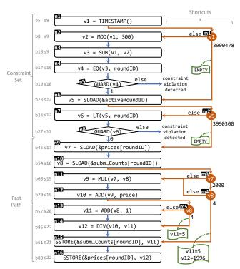
**Figure 17.** Accelerated program of  $Tx_e$  synthesized in FC3. All the variables whose names do not start with v, such as roundID, &activeRoundID, are constants. The corresponding line numbers in EVM trace and the source code are annotated in the left two columns.
