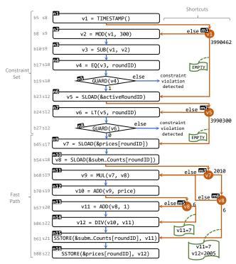
**Figure 16.** Accelerated program of  $Tx_e$  synthesized in FC2. All the variables whose names do not start with v, such as roundID, &activeRoundID, are constants. The corresponding line numbers in EVM trace and the source code are annotated in the left two columns.
