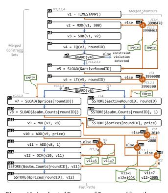
**Figure 10.** Accelerated Program of  $Tx_e$  merged from the synthesized programs in FC1, FC2, FC3, and FC4, with the source APs of the merged instructions and shortcuts annotated.
