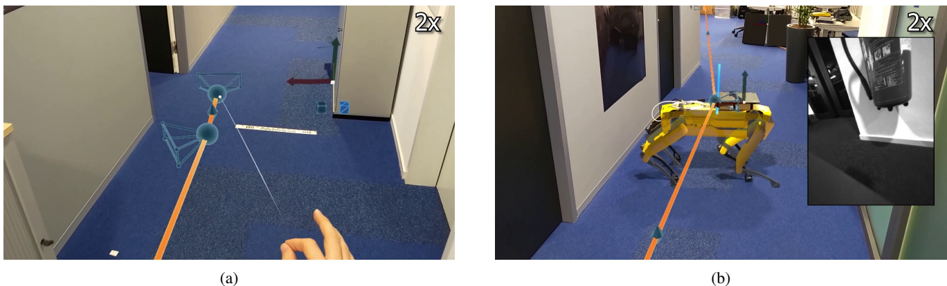
Fig. 2: Mission planning and execution. Fig. 2a shows the view through the HoloLens as the user moved holographic markers for the trajectory waypoints. Each waypoint is represented by a sphere for the desired position, and a camera frustum to define the orientation the robot should take for inspection. The axes to the right of the trajectory mark the origin of an automatically-created spatial anchor coordinate system. Fig. 2b shows the user's view as the robot is executing the mission, with a robot model overlaid on the physical one, and a sample data capture at an inspection pose. This user view during mission execution is only for illustration, as the robot can execute the missions autonomously without human intervention.
