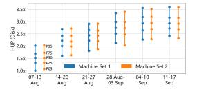
Figure 4: Disk HUP for a cluster in South America (of 450 servers) during Aug-Sep 2021: The (normalized) percentiles drift across weeks (1% - 32%) significantly; but they vary much less (1% - 2%) across the two disjoint server sets.
