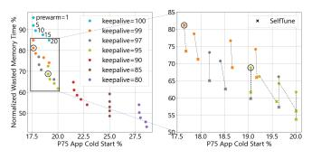
Figure 7: Performance of the VM management policy [54] on AzureFaaS data: (left) sweep of prewarm and keepalive, fixed for all apps; circled dots are the choices recommended in [54]; (right) with SelfTune for tuning the two parameters for each app, and memory wastage as reward; the dots are the starting points for SelfTune, and the corresponding crosses indicate the performance at convergence.
