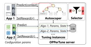
Figure 1: OPPerTune service architecture. Applications create *tuning instances* on the server to tune various configuration parameters. *Autoscoper* helps automatically create, manage, and scope tuning instances based on the application's dynamic context. *Selector* helps pick the most promising configuration parameters to tune.
