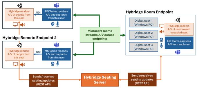
Figure 6: System diagram for the Hybridge prototype showing connections between various parts of the system.
