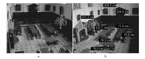
**Fig. 11.** Estimating the heights of points from two views of The Queen's College dining hall. The heights of the reference points, shown black on white, were measured by hand  $(\pm 0.5cm)$  to be 76cm (table top), and 230cm (fireplace). The step was computed to be 11.4cm high and measured by hand as 11.0cm.
