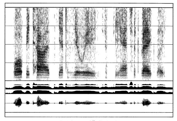
Fig. 5. Spectrogram of  $H_{\infty}$  filtered speech.
