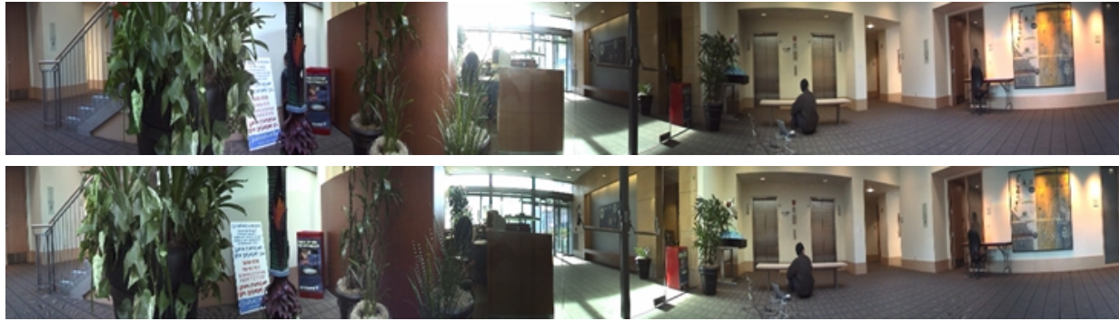
Figure 8: Dual-strip images formed by moving a single perspective camera 360^\circ on a circle and building mosaics from the 60th column (top) and 260th column (bottom) of the input image sequence.
