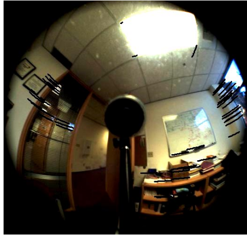
Figure 4: Example of tracking for office scene: 100 feature tracks are superimposed on the first omnidirectional frame.
