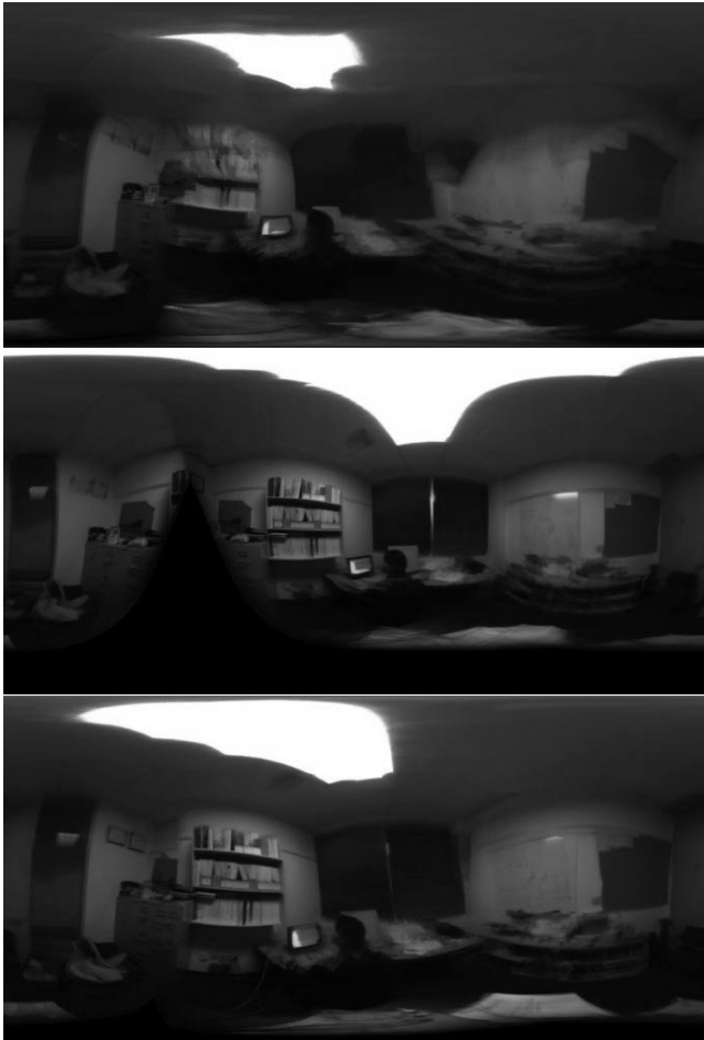
Figure 7: Results of mosaicking. Top: Using circle-based parameters, Middle: Using algebraic error, Bottom: Using image error (proposed).
